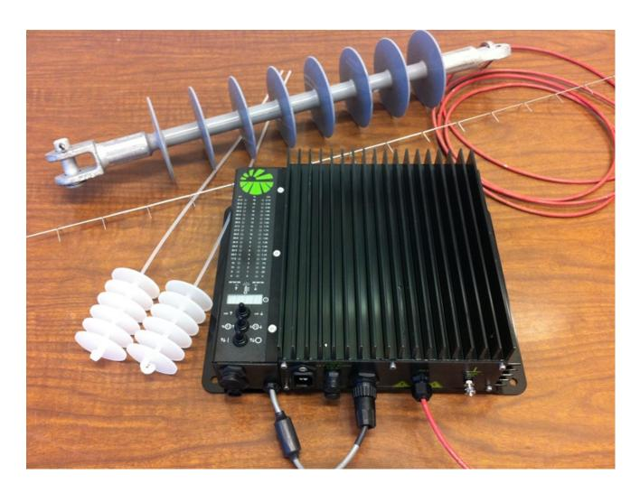
The basic components of the EPI System have no moving parts. A power supply, specially designed to withstand a corrosive environment, delivers ions under "high-pressure" into the air through stainless steel corona points. The corona line is insulated from a ground via insulators.
